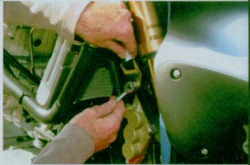
Above Hamby cinches down the front end of the 'Busa using an MPS lowering strap, to bring the bike closer to the ground and lessen the chance of it rearing up on the rear wheel under a hard launch.
