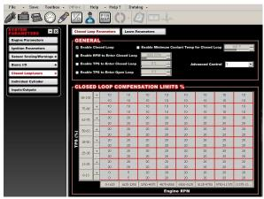
The ECU has closed loop compensation limits that are set in the closed loop compensation table. This is where you tell the ECU how much fuel as a percentage it can either add or remove from the base fuel table at a given throttle position or MAP sensor pressure. For example: at idle, you could only allow the closed loop compensation to remove 5% and add 0%, but at 100% throttle position at 10,000 rpm you may have +40%
