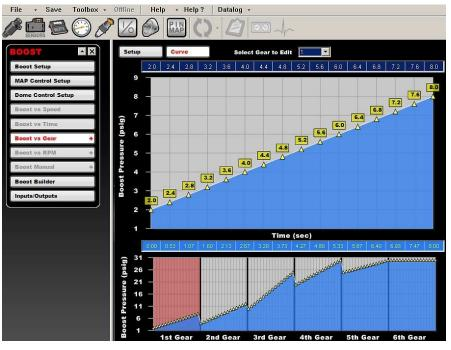
The Boost Controller compares with stand alone controllers costing as much as the HP ECU. The first thing you will need to determine what type of wastegate you are using. This will either be a single port or the preferred dual port type wastegate. You will need one 3
