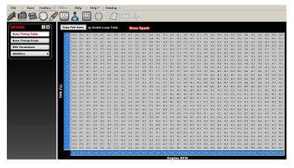
The base ignition table has an RPM axis and either a TPS (throttle position sensor) or MAP (manifold air pressure) axis just like the fuel table. The values in this table are the number of degrees before TDC to fire the spark plugs.
