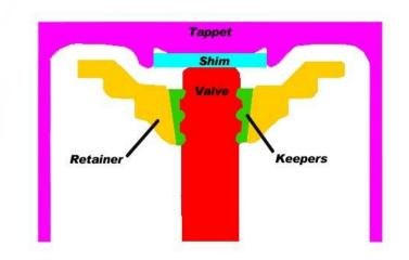
Shim in Tappet with Triple Groove Keepers
