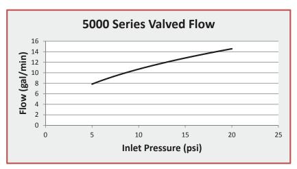
Jiffy-tite Quick Connect Fluid Fittings using standard stoddard solvent with a specific gravity of .750 and 80° fluid temperature through a -10AN hose. Refer to page 25.
