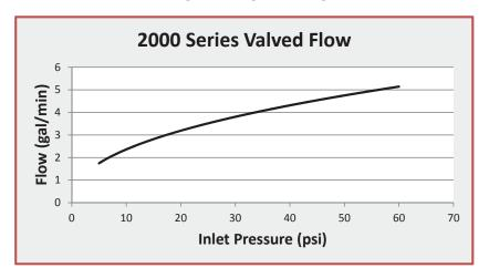
Jiffy-tite Quick Connect Fluid Fittings using standard Stoddard solvent with a specific gravity of .750 and 80° fluid temperature through a -6AN hose. Refer to page 6.
