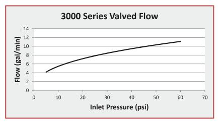
Jiffy-tite Quick Connect Fluid Fittings using standard stoddard solvent with a specific gravity of .750 and 80° fluid temperature through a -8AN hose. Refer to page 16.
