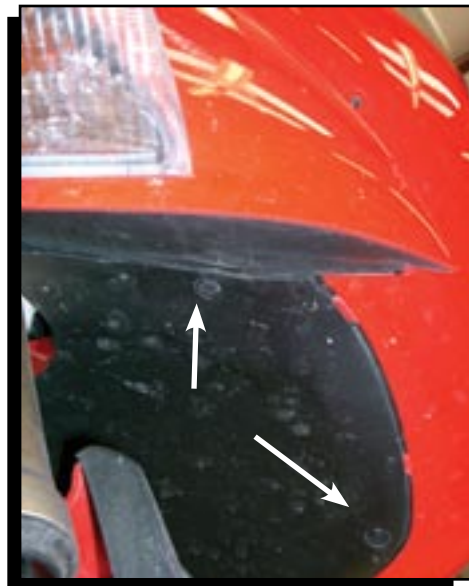
Figure 4 Removing the Headlight Panels.
