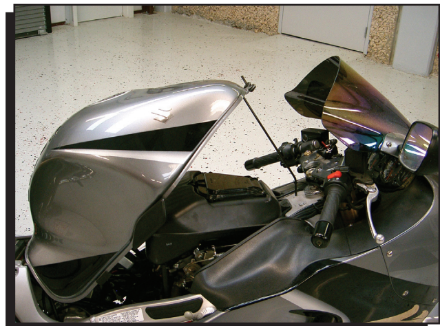
Figure 2 Propping the Fuel Tank.
