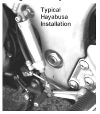
**Mount Air Bottle, Electronic Kill & Electric Air Valve** – Every brand and model bike is different, so you will need to fabricate your own bottle mounting. Make sure they are fastened securely. The Electronic Engine Kill & Electric Air Valve can be mounted anywhere using zip ties, double sided tape, or Velcro strips. Generally the best spot for both components is in the tail section. We offer a remote air gauge mount kit to mount the gauge away from the tank if desired.
