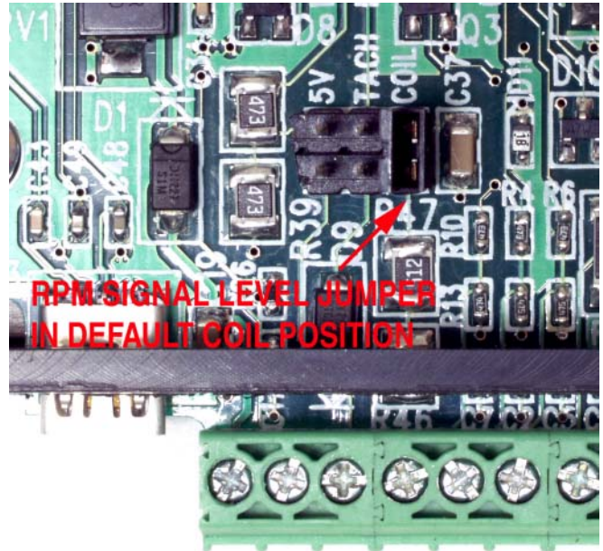
Figure 13 – RPM Signal Level Jumper
