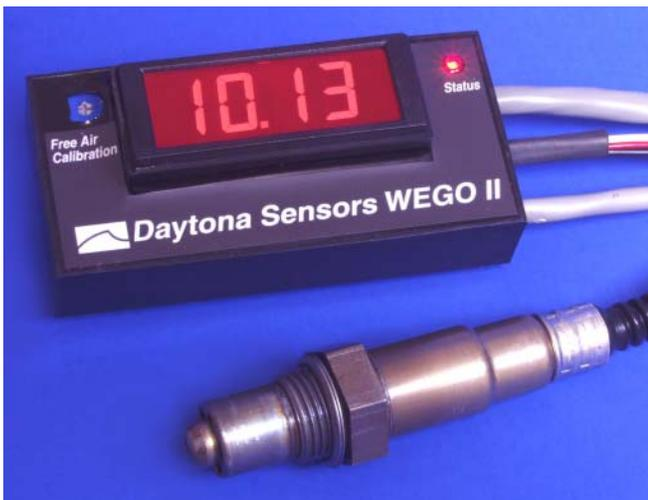
After installation, the WEGO II system requires free air calibration. This should be done with the sensor dangling in free air. The environment must be free of hydrocarbon vapors. We suggest that you perform the free air calibration outdoors. Turn the free air adjustment trimpot on the WEGO II full
