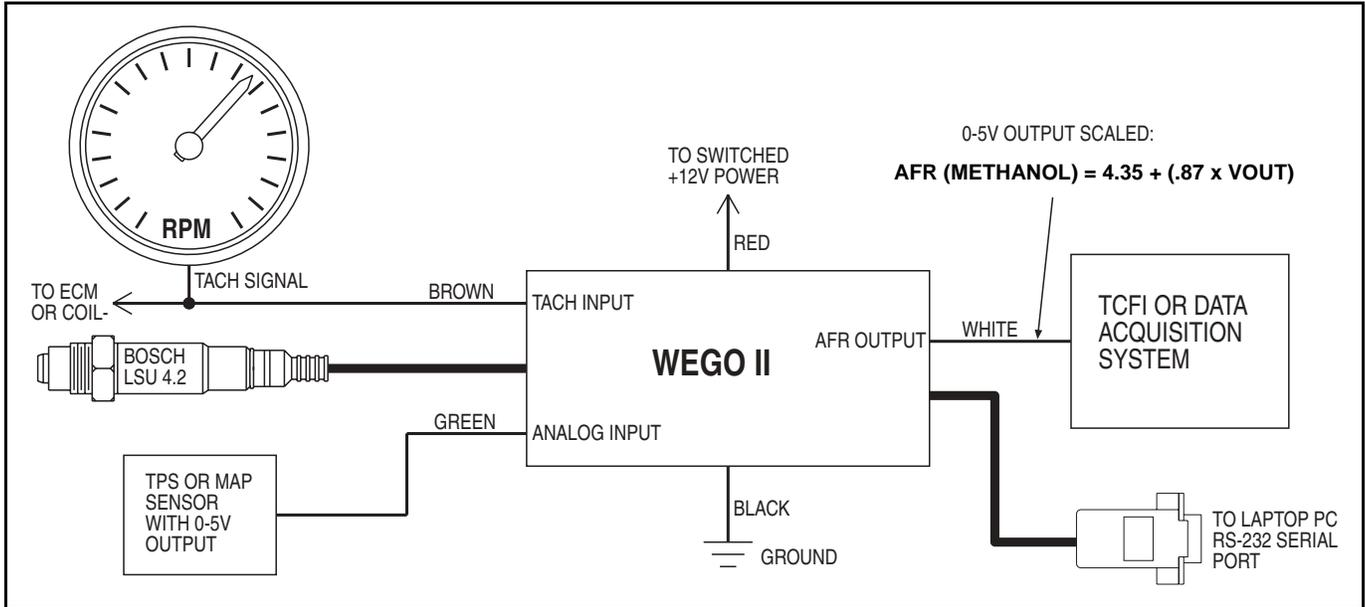
8. Optional signal hookups, including engine RPM and analog signal data logging, are explained in sections 9-11. If you are not using these features, tape up the brown, green, and white wires.
