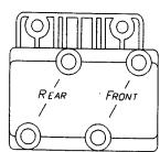
DC6-4 (FOUR TOWER) FOR DUAL SPARK PLUG APPLICATIONS
