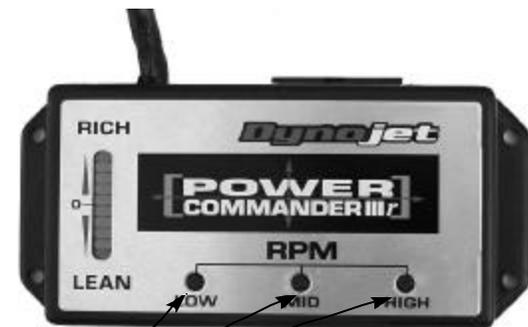
Hold these buttons and turn the ignition on to adjust the Power Commander
