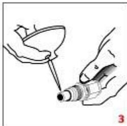
3. Lubricate the inside of the hose, the cutter threads and the socket threads with Earl's assembly lube or engine oil. Place the nipple in a vise.
