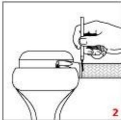
2. Place the socket in a vise and insert the end of the hose into the socket until the hose butts against the bottom of the threads provided for the cutter. Gently pull the hose back until there is a 1/16" to 1/8" gap between the end of the hose and the bottom of the threads-mark hose at bottom of socket with a felt pen so that you can detect any tendency of the hose to be pushed out as you complete the assembly.
