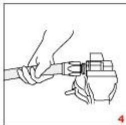
4. Holding the hose and not the socket, push the hose and the socket onto the nipple until the socket threads can be started on the cutter. Holding the hose and not the socket, start the threads and go as far as you can by hand. Depending on the size of the hose, some force may be necessary in this part of the operation.
