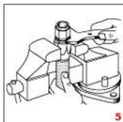
5. To complete the assembly it doesn't matter whether the nipple or the socket is held in the vise. Holding one or the other in the vise and using a suitable wrench on the other, tighten the socket onto the cutter threads until the socket is within .060" of
