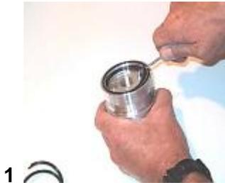
Use a small screwdriver to gently pry up the top end of the metal spirol lok that holds the filter in the case.
