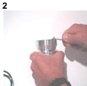
Use caution not to damage the rubber quad-ring that seals the top of the filter to the engine (it can be removed if you like).
