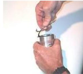
Pull the spirol lok up and toward the center of the filter in a circular motion and work the spirol lok out of its slot. You should now be able to remove the filter element from the case.
