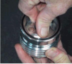
2. Gently push the filter element straight down into the housing.
