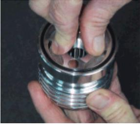
3. Twist filter element 1/3 turn counter clockwise (to the left)
