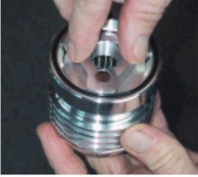
4. Release the filter element. It should spring up through the 3 slots in the filter housing. You can now remove the filter element for inspection and cleaning
