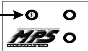
vary from bike to bike. It's generally better to start with too much kill time and work your way quicker. We generally start at around 75 ms. of kill time. The Kill Time is adjusted via a small potentiometer accessed through the grommet on the front of the unit. Using a small screwdriver Carefully turn the pot
