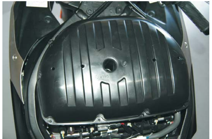
Figure 5 Remove Air Filter box
