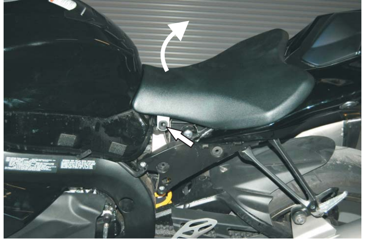
Figure 1 Remove bolts lift seat
