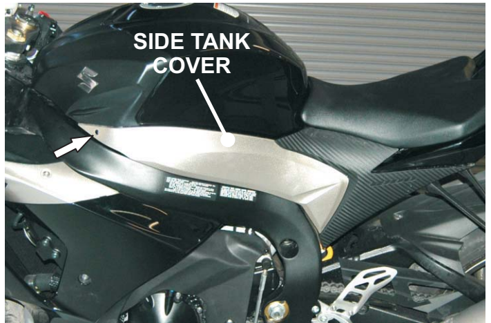
Figure 2 Remove tank cover panels
