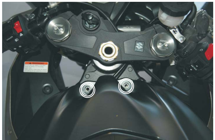
Figure 3 Remove tank bolts
