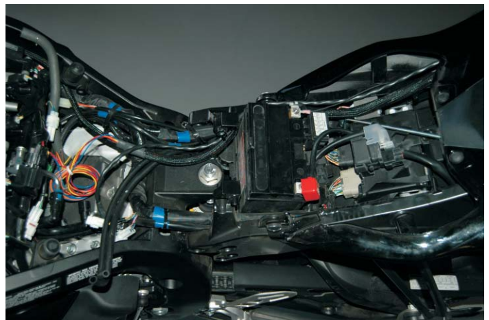
Figure 6 SB6 Harness routing
