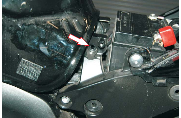
Figure 4 Remove tank bolt & tank
