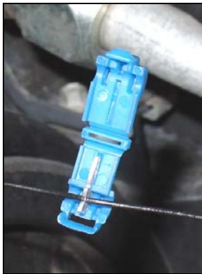
Figure 4 (T-Tap connector installation)
