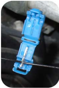
Figure 3 (T-Tap connector installation)
