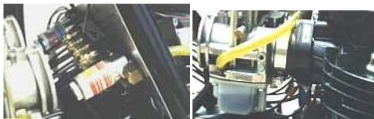
The MPS Nitrous Distribution Block (left) and The MPS Nitrous Manifolds (right)
