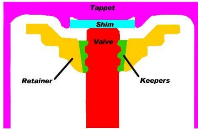
**Shim in Tappet with Triple Groove Keepers**
