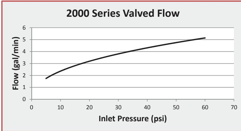
Jiffy-tite Quick Connect Fluid Fittings using standard Stoddard solvent with a specific gravity of .750 and 80° fluid temperature through a -6AN hose. Refer to page 6.
