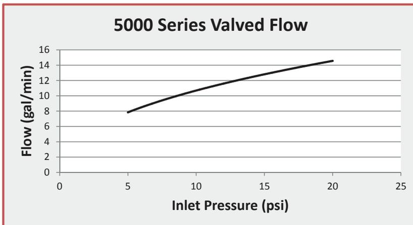
Jiffy-tite Quick Connect Fluid Fittings using standard stoddard solvent with a specific gravity of .750 and 80° fluid temperature through a -10AN hose. Refer to page 25.
