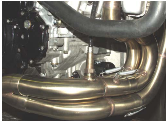
Figure 6 – Bosch Sensor Installation
