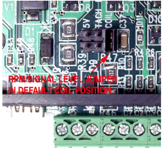
Figure 13 – RPM Signal Level Jumper
