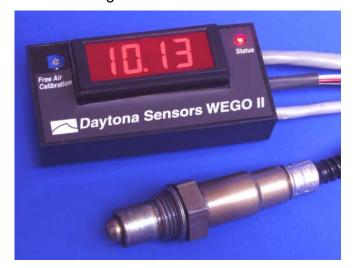
After installation, the WEGO II system requires free air calibration. This should be done with the sensor dangling in free air. The environment must be free of hydrocarbon vapors. We suggest that you perform the free air calibration outdoors. Turn the free air adjustment trimpot on the WEGO II full
