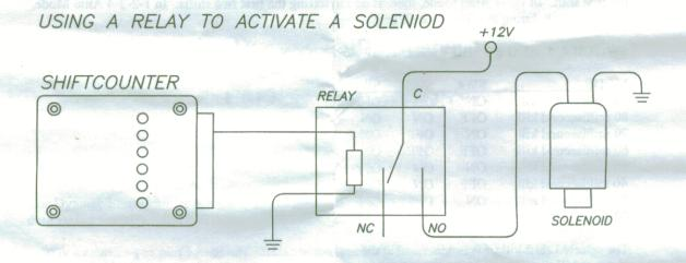
NOTE — THE SHIFT COUNTER OUTPUTS SUPPLY +12 VOLTS WHEN ACTIVATED.
