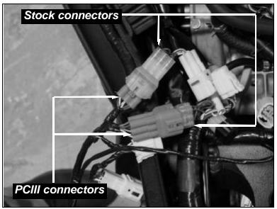
6 Plug the TPS connectors from the PCIII (white connectors) in-line of the stock wiring harness (Fig. C).
