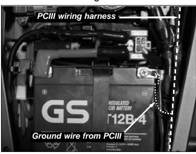
8 Install the PCIII in the rear section of the trunk using the supplied velcro (Fig. E). Make sure to clean both surfaces first with alcohol.
