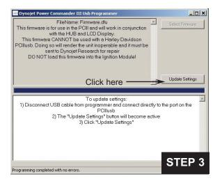
3 Unplug the USB cable from the programmer and plug it directly into the USB port of the Power Commander.
