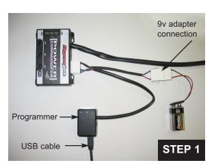
1 Connect your USB cable to your computer and then to the programmer. Connect the 9v battery adapter to the programmer.
