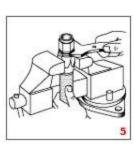
bottoming on the nipple. Do not use an adjustable or over-size wrench or you will damage either the nipple or the socket.
