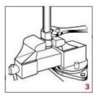
**NOTE**: Tube-Mate hose ends are designed to be used only with beaded, barbed or grooved rigid tubing at no more than 25 psi working pressure.
