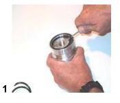
Use a small screwdriver to gently pry up the top end of the metal spirol lok that holds the filter in the case.
