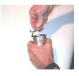
Pull the spirol lok up and toward the center of the filter in a circular motion and work the spirol lok out of its slot. You should now be able to remove the filter element from the case.
