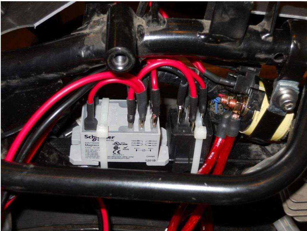
2. On the left side of the tail section, remove the plastic cover that protects the starter solenoid. Disconnect the starter cable from the starter solenoid (lower cable) and the starter. Remove the cable from the bike. Save the black plastic boot that covers the starter nut/bolt. You will re-use it when connecting the new starter cable. Connect the ground cable from the secondary battery to the open (lower) position on the primary starter solenoid.
