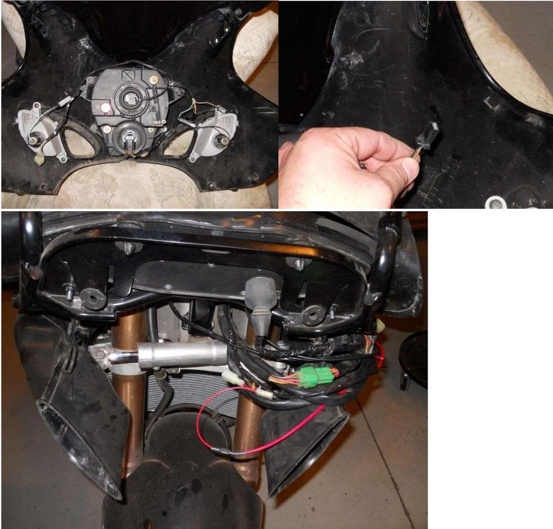
9. With everything connected, you can now test the system. The main battery/charging system will only charge the secondary battery with the key on. Under heavy use with little charging, you may need to charge the secondary battery between rounds (drag racing) but should not need charging under normal use. Ensure that all loose wires are tied and secure before re-installing the body on the bike.
