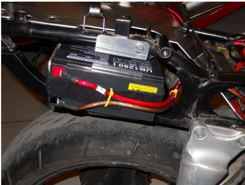
6. Route the wires labeled Clutch and Ign. Switch forward following the main wire loom. At this point, it is recommended to remove the front nose fairing of the bike. This will allow an easier and cleaner installation. You can use zip ties to secure the wires along the loom for a clean look.
