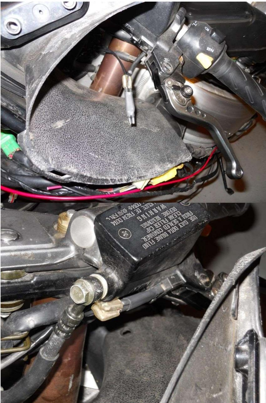
8. Now you will need to connect the Ign. Switch wire to the "Euro" connector located behind the headlight. It will be located on the right side of the headlight harness. It has a factory end on it as to allow for other accessory items to still be utilized.
