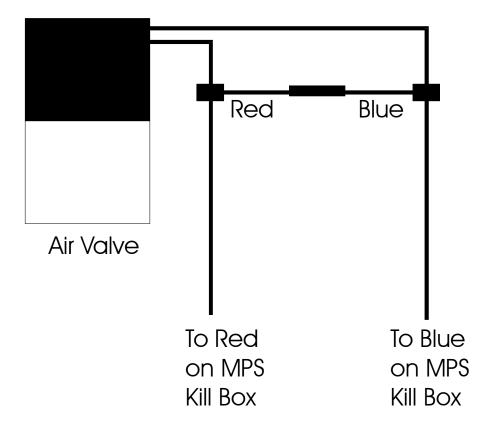
The MPS Air Valve Diode is to prevent voltage spikes that activate the kill a second time when the air valve coil is discharged. To prevent the unwanted double kill install the diode as shown below.
