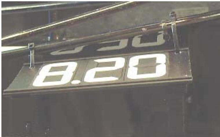
Find a good spot to mount your dial in boards. Using the Velcro provided, stick a couple strips to each side of the dial in boards. Stick the dial in boards to where you want them. Then you will need to drill a small hole in each side to zip tie them. This will provide a pivot so you can flip the dial in board up to change the digits and a secure means to hold them on if the Velcro loosens.
