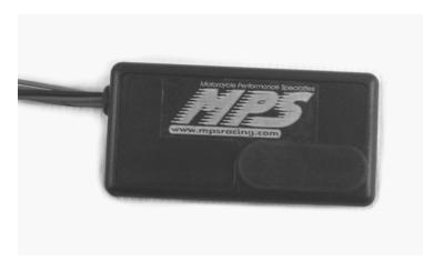
The MPS Fast FI Mixture Control P/N 1-0337 is a simple means to adjust the fuel curves on your fuel-injected motorcycle. This allows for tuning after the installation of aftermarket exhausts, intake modifications, or internal motor modifications. It can only richen the fuel mixture. It cannot lean the mixture. The Fast FI Mixture Control has a low speed pot that adds fuel at low speed much like a mixture screw on a carburetor. The
