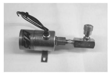
Run one line from the master Cylinder to the side of the Hydraulic Clutch Release that has the needle valve. All threads are 1/8 NPT female. The second line will go from the slave cylinder to the side of the Hydraulic Clutch Release labeled brake.
