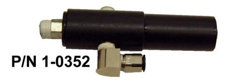
The pin valves on CO2 bottles operate like schrader valves on a tire. Pushing down the pin opens the valve. The pin valve actuator works by pushing down on the pin when you screw the on-off knob clockwise. Since CO2 is a liquid in the bottle and the regulator can't regulate liquid, you must mount the bottle so that only gas and no liquid can get into the regulator. To install and set up the MPS Paintball Regulator assembly follow the directions below.
