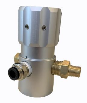
The MPS Pressure Regulator has 4 ports. A 1/4" NPT inlet (High Pressure) port, a 1/4" NPT outlet (Regulated Pressure 0-600psi), a 1/8" NPT gauge (Regulated Pressure 0-600psi) port, and a 1/8" NPT gauge (High Pressure) port. The ports are all labeled, HP for high pressure and LP for low or regulated pressure.
