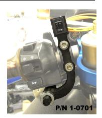
Remove the stock clutch master cylinder bolts. Using the stainless steel bolts and washers provided, bolt the Street Lite Single Switch and factory clamp to the master cylinder. Tighten to factory specs. Do not remove factory master cylinder clamp! The Street Lite Tether Kill Switch does not replace the stock master cylinder clamp!
