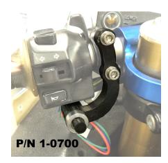
Remove the stock clutch master cylinder bolts. Using the stainless steel bolts and washers provided, bolt the Street Lite Single Switch and factory clamp to the master cylinder. Tighten to factory specs. Do not remove factory master cylinder clamp! The Street Lite Tether Kill Switch does not replace the stock master cylinder clamp!
