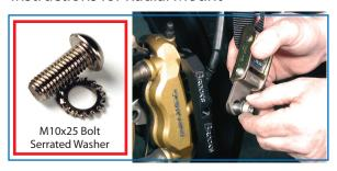
Bolt Strap End to Brock's Radial Mount Strap Bracket Kit using M10x25 Bolt and Serrated Washer supplied with kit.
