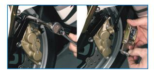
Remove top bolt from front brake caliper.
