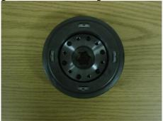
Install the new pressure plate from the kit and then the snap ring.
