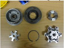
Install the diaphragm springs into the pressure plate.
