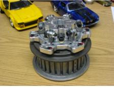
Check the distance between the bottom of the lockup and the top of the pressure plate. Ideally there should be .100-.125 inch clearance between the lockup and the pressure plate. This distance is controlled by the clutch pack stack height.
