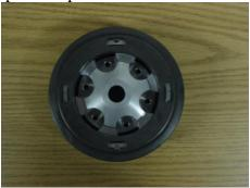
Install the lockup unit onto the flange and tighten it up.
