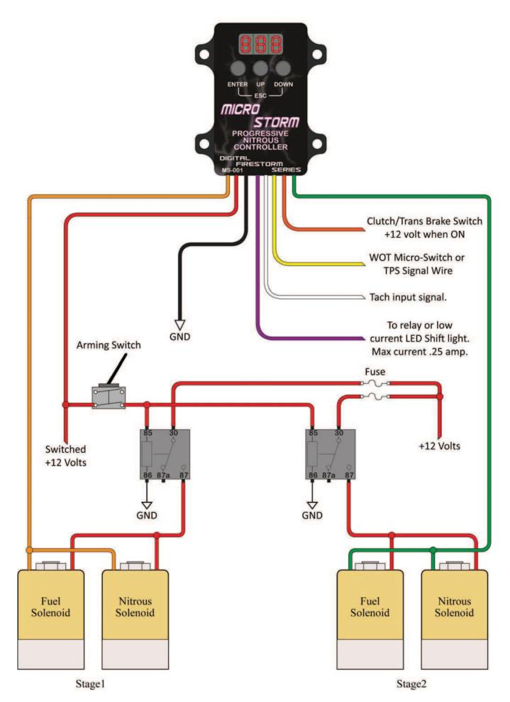
**Battery Ground**, the best place to connect the Black, 16 ga wire is directly to the battery negative terminal. If this is NOT possible then the connection should be to the frame. There MUST be a quality, large diameter ground cable going from the battery negative terminal to the frame if the frame connection method is used.
