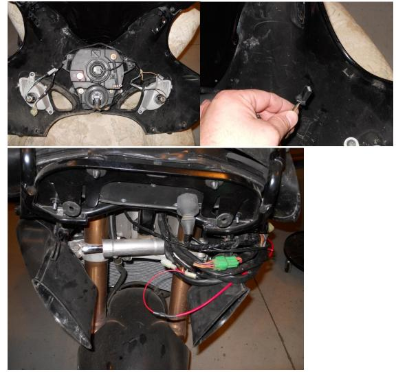
9. With everything connected, you can now test the system. The main battery/charging system will only charge the secondary battery with the key on. Under heavy use with little charging, you may need to charge the secondary battery between rounds (drag racing) but should not need charging under normal use. Ensure that all lose wires are tied and secure before re-installing the body on the bike.
