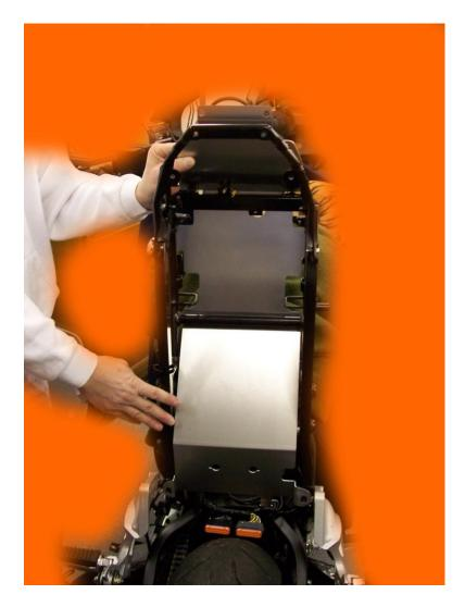
11. Now attach the inner fender to the sub frame as shown with the 2 front shouldered mount bolts.
