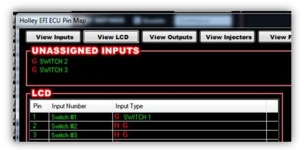
5. Select 'View Outputs' from the 'Pin Map' and drag the outputs to the pin location the device was wired to.
