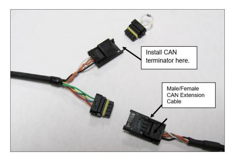
Holley EFI main harnesses use two types of CAN connectors. Earlier harnesses use a 2 pin metripak connector. The kit includes an adapter to go from this to the 4' extension harness (note the white power and black ground wires are NOT needed for the Pro Dash, but need to be connected if other CAN devices require it for their power supply). Later harnesses plug directly into the 4' extension harness.
